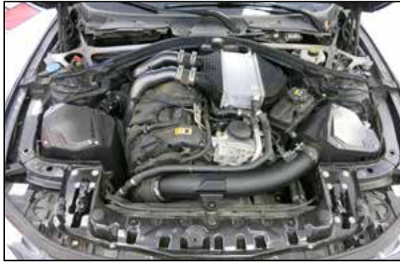
34. Reinstall the Strut tower brace, cowl covers and engine cover.
