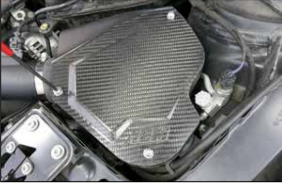
33. Install the carbon fiber air filter covers.
